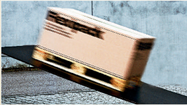
Not using anti-slip interlayers (AntiRutsch): sliding friction coefficient < 0,2 \mu\text{D}
